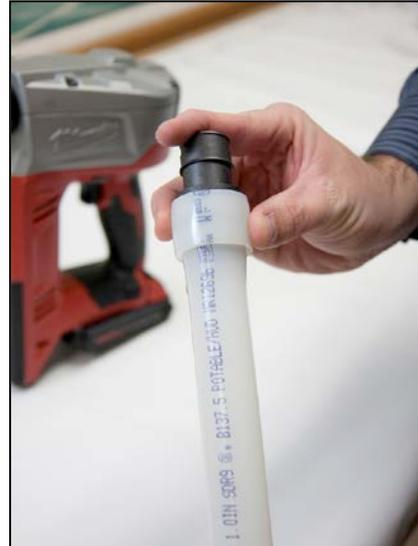
**Using engineered polymer (EP) fittings in a residential multipurpose fire sprinkler design can reduce the overall list price on an average system by as much as 10 percent.**
